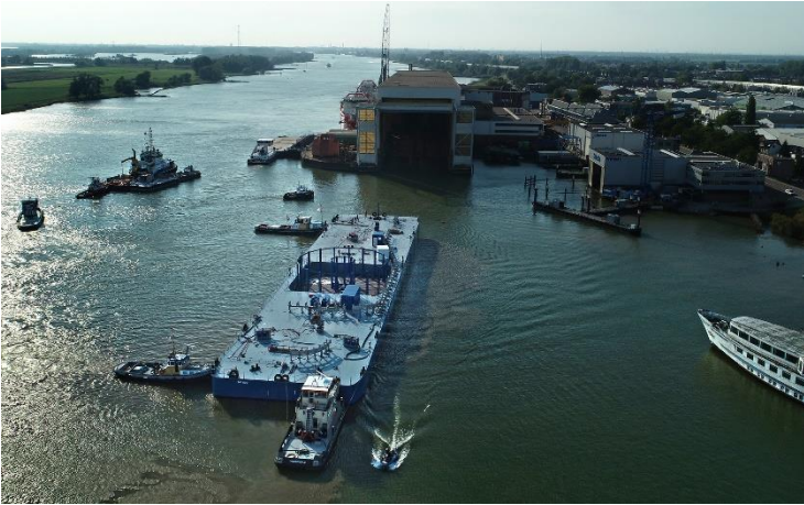
The barge was launched at the Neptune Marine shipyard in Hardinxveld in the Netherlands and has been designed with integrated cable carousel to offer NKT the opportunity to carry several thousand tonnes of cables. Photos: Neptune Marine
