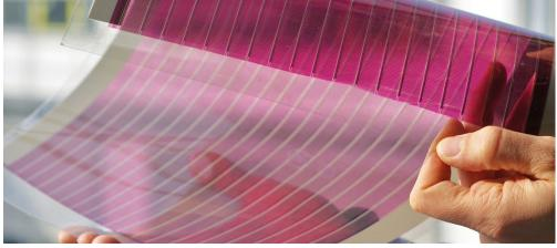
Flexible, transparent organic solar PV modules can open up new fields of application. © Fraunhofer ISE
