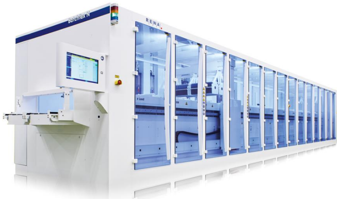
Image 2: Texturing solar cells in the BatchTex XL machine
