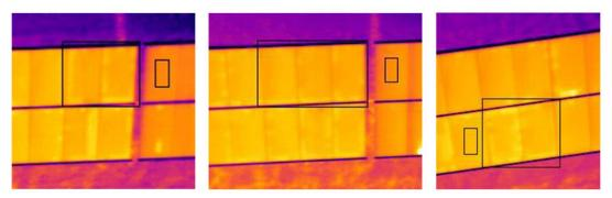
SOLAR PV MODULES IDENTIFIED WITH PID USING AERIAL THERMOGRAPHY © ABOVE
