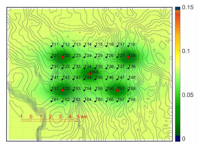
Figure 3. One of the case studies illustrating the importance of full-field coverage: the certainty of Hs measurement degrades as standard deviation increases with distance from sensors
