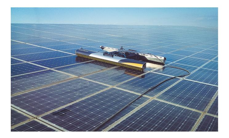
solution described above, but other solutions are already in place, such as large tractormounted brushes. When the distance between rows of panels is sufficient, this solution offers the advantage of quick cleaning with a single brush and an operator who moves from one row to another by tractor. However, this solution depends on the availability of the solar panels in sufficiently spaced rows, on human presence
