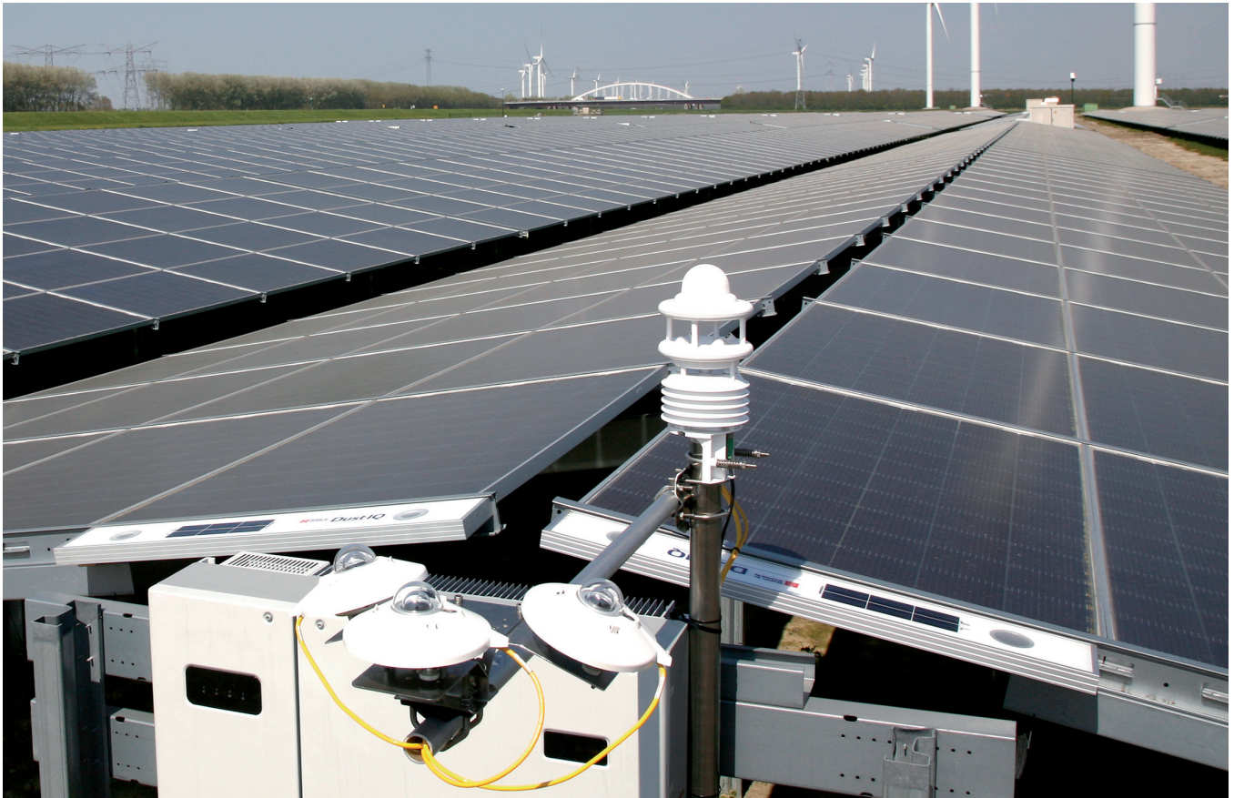
Class A monitoring system: GHI and POA pyranometers, weather station, soiling monitors
