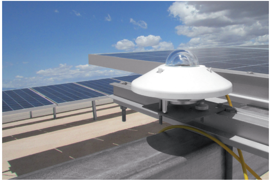
Pyranometer measuring plane of array (POA) irradiance
