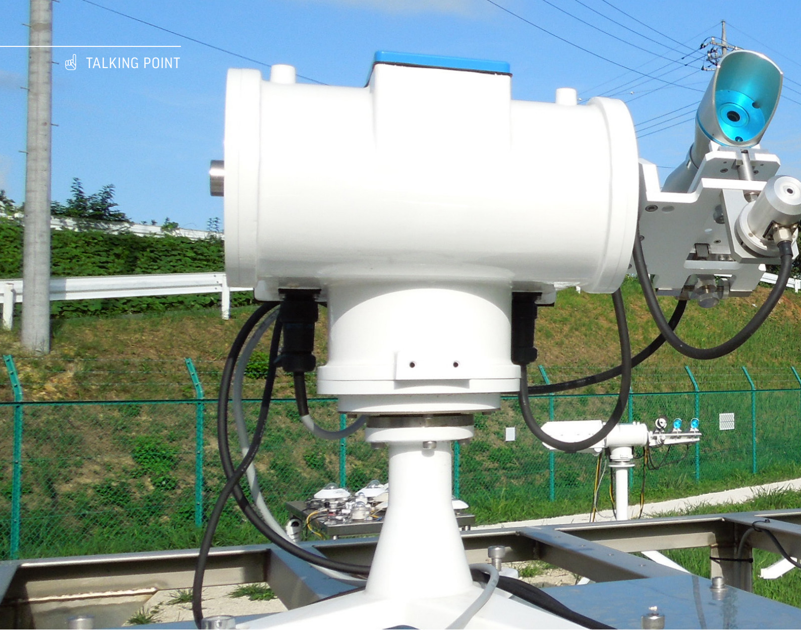
STR-21G Sun Tracker with MS-57 Pyrheliometer next to the MS-90 DNI Sensor at EKO Instruments Ami Solar Park, Japan
