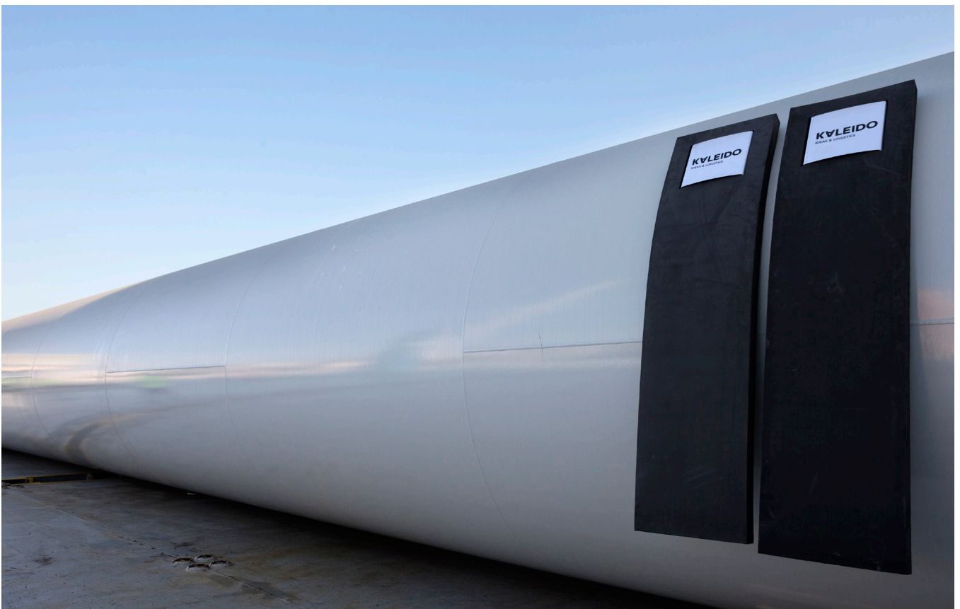
Magnet Foam, a safety system to protect tower sections.
