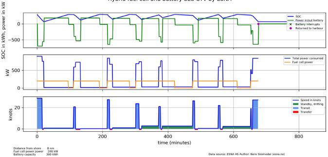
Trip duration= 676 minutes = 11:16 h Sum energy consumed= 1968.1 kWh Max power= 900.9 kW Minimum power= 15.2 kW Average power usage= 174.7 kW Max speed= 28.7 kts Average speed= 4.0 kts Sailed distance = 44.76 nm with 8 transfers Energy produced by FC= 1736.7 kWh, i.e. approx 104 kg of H2 Specific fuel cons 60.1 g/kWh Battery SOC at start 300.0 kWh Battery SOC at finish 68.6 kWh Minimum battery SOC= 66.6 kWh Number of interrupts= 0 at []
