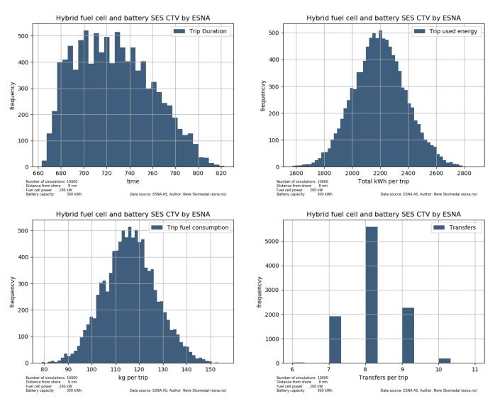
Figure 5. Frequency plot of trip duration, total energy usage, kg H2 used in the fuel cell and number of transfers completed.
