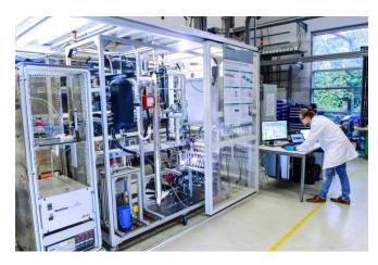
Scale-down miniplant for research on methanol synthesis at Fraunhofer ISE. ©Fraunhofer ISE
