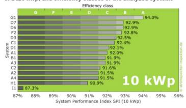
Fronius Symo GEN24 10.0 Plus and BYD Battery-Box H11.5 (G1) are the only systems to achieve efficiency class A with a maximum value of 94%, which has never been achieved before.
