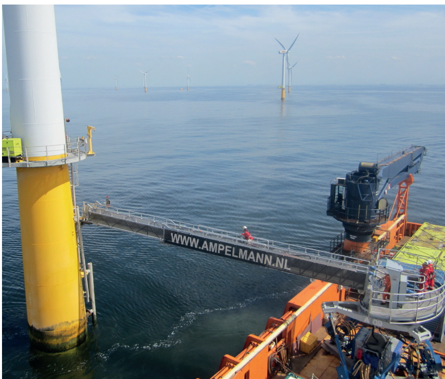
Ampelmann A-type in operation
