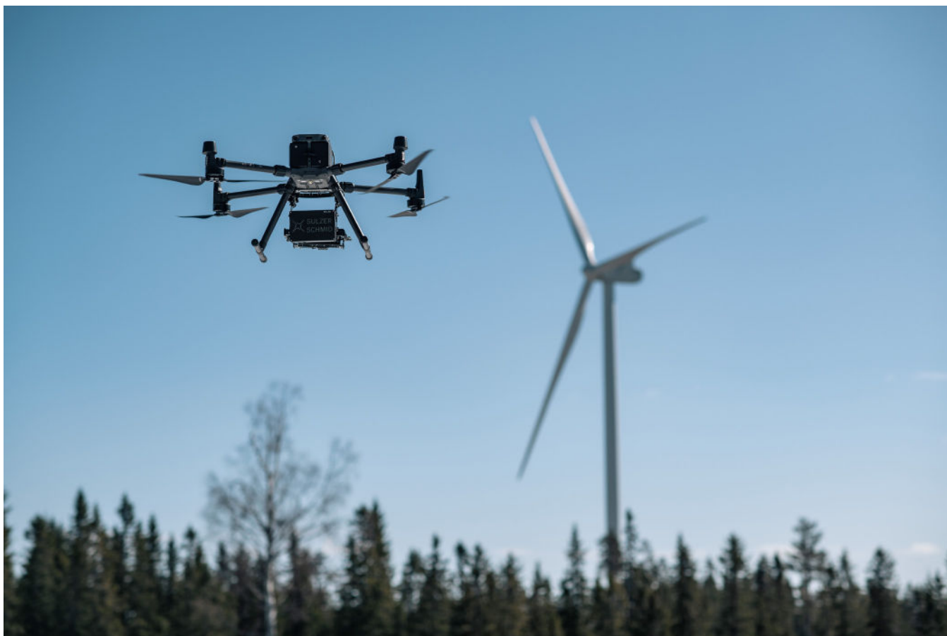
High-quality rotor blade data is obtained with digital inspection methods
