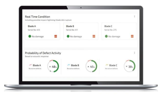
NDE 4.0 technologies like Sensoria™ collect real-time integrity data and report it through an online, easily-accessible data portal, enabling wind turbine operators to proactively plan their inspection and maintenance activities based on the actual conditions of their assets
