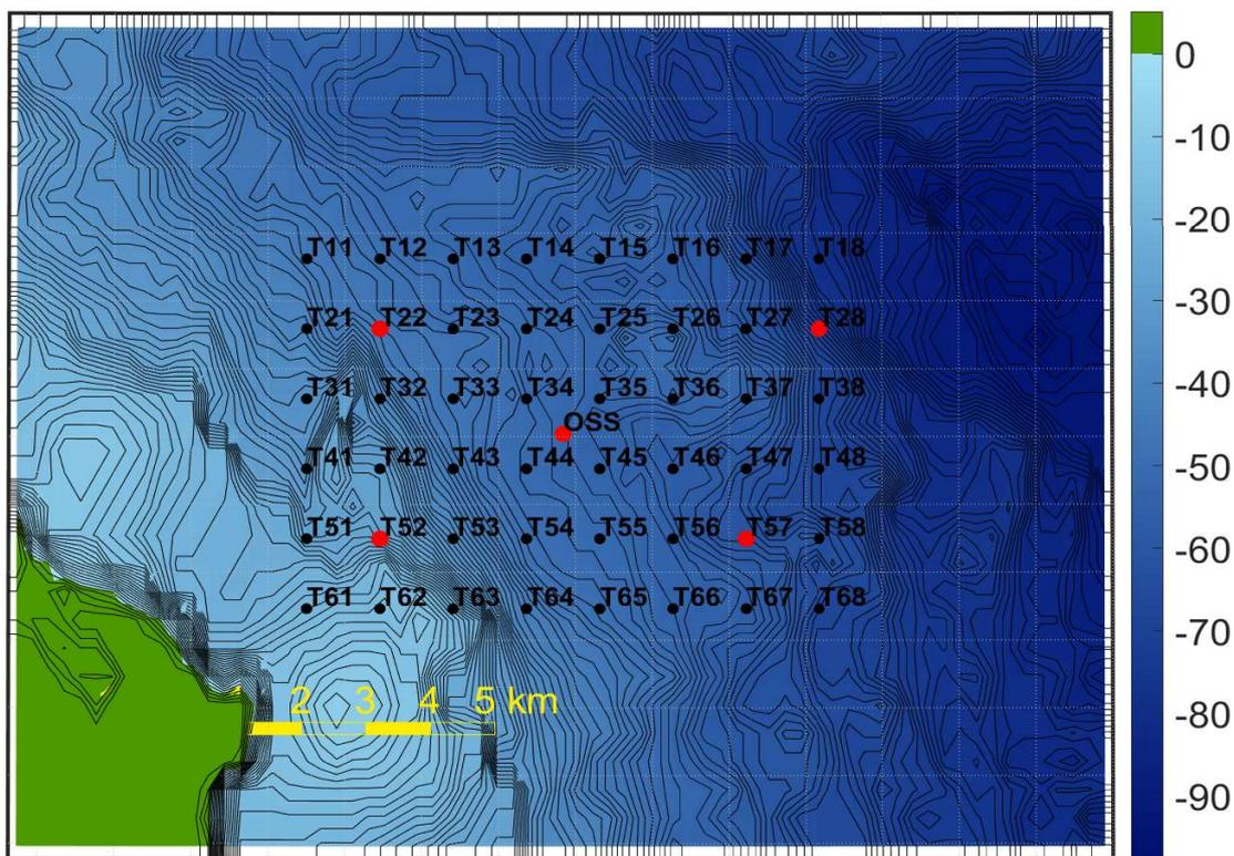
Figure 1. Site bathymetry: 1m contours
