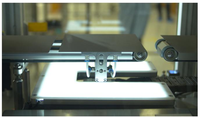
Manufacturing HJT cells requires significantly fewer production steps compared to TOPCon, six versus 11 to 14 respectively, and REC's special low temperature production process for HJT cells significantly reduces energy consumption, helping to better protect the environment.
