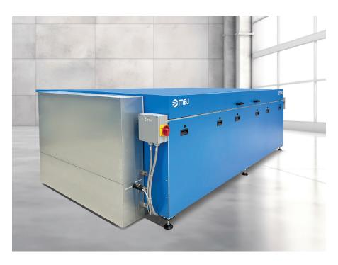
The Steady State Sun Simulator is optimized for cell and mini-module testing. With 22 LED types, it reaches 98% spectral coverage and a deviation of 24.2%. It offers steady illumination and allows combined use of different spectra for soaking and measurement within a single test recipe.
