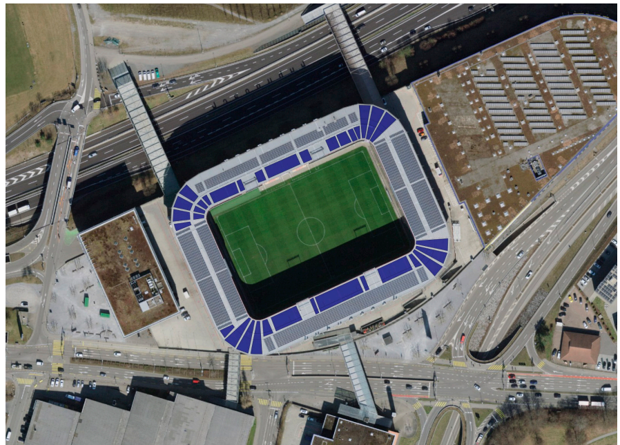
In the illustration, the previous solar system is recognizable by the grey module fields, the blue areas represent the fields that should be added
