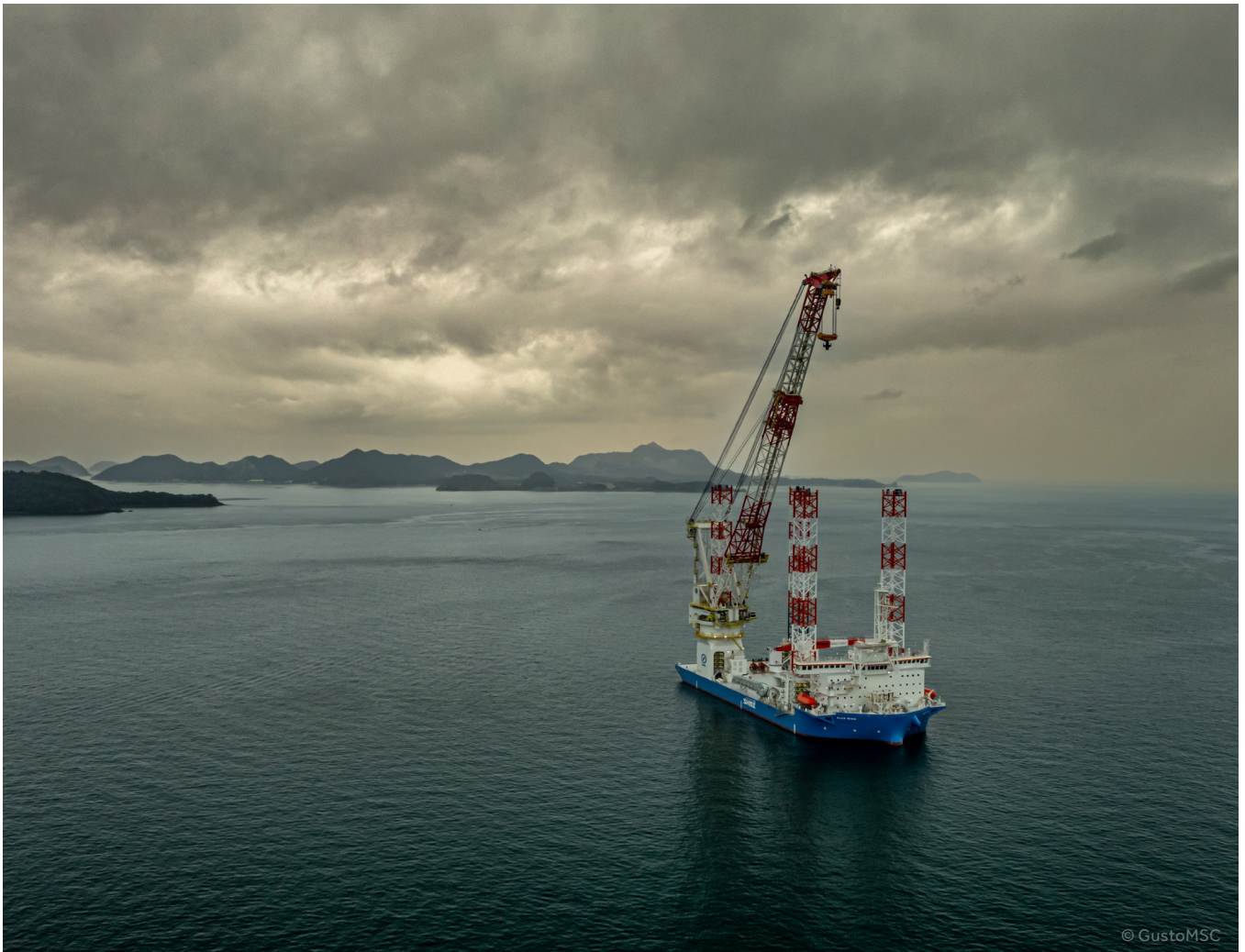
Shimizu Corporation's Blue Wind, a GustoMSC-designed SC-14000XL wind turbine installation vessel, operating off Japan's coast
