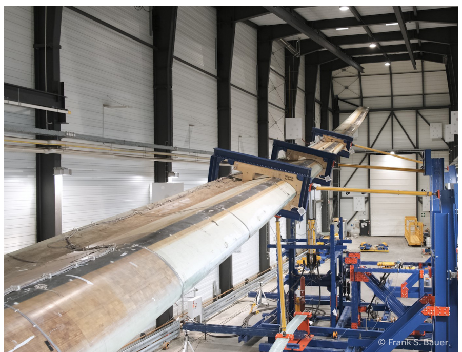
Bi-axial blade test in one of Fraunhofer IWES' test benches
