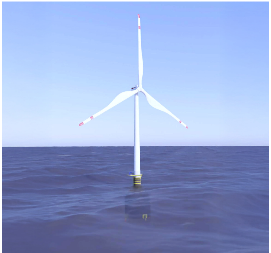
ECO TLP provides high static vertical stability to ensure maximum power generation and minimizes motion experienced by the nacelle to allow constant and reliable power generation
