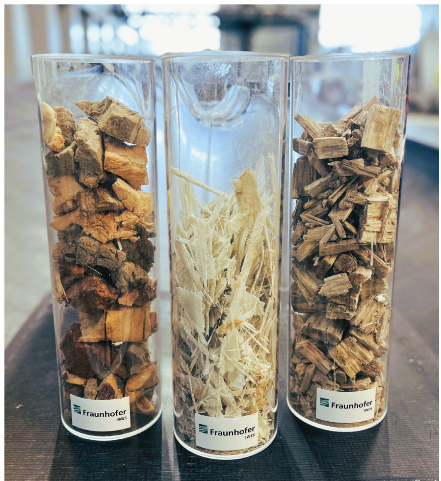
Following separation: the shredded PVC foam, GFRP and balsa wood from a rotor blade © Fraunhofer IWES
