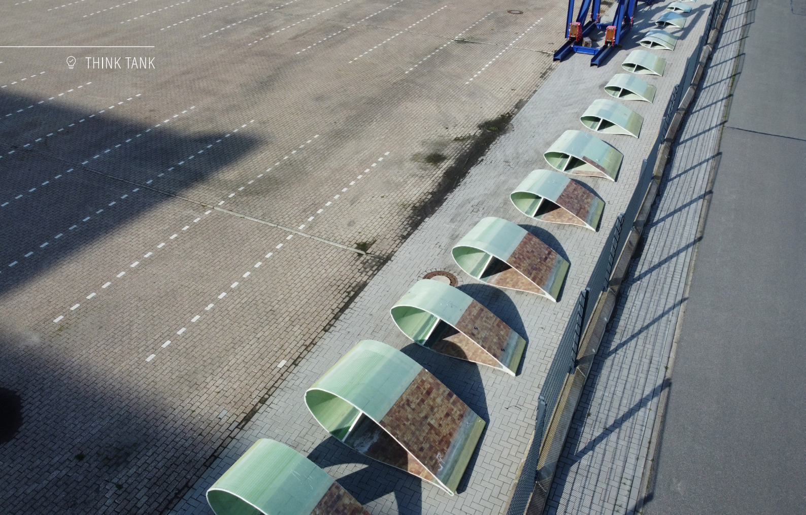
Rotor blade cut into cross sections © Fraunhofer IWES
