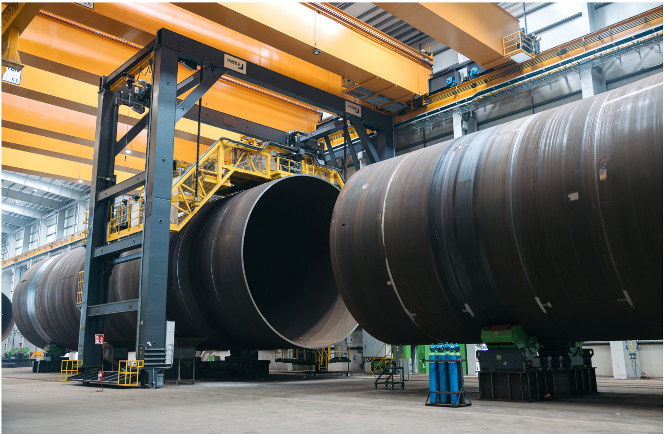
Modern wind towers contain kilometres of weld seams, requiring highly consistent welding processes during fabrication
