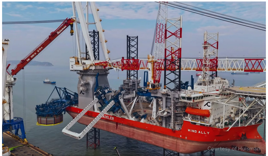
Wind Ally: engineered to transport five monopiles of up to 12 m diameter per trip, showcasing the complex integration of the crane, jacking system, and Huisman foundation handling equipment required for safe and efficient installation
