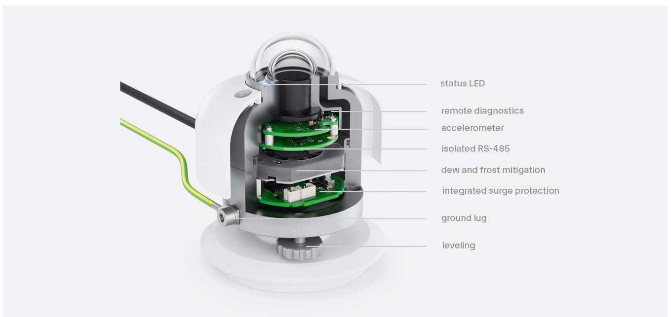
A cut through of the SR300-D1 industrial Class A pyranometer showing the different components inside the instrument
